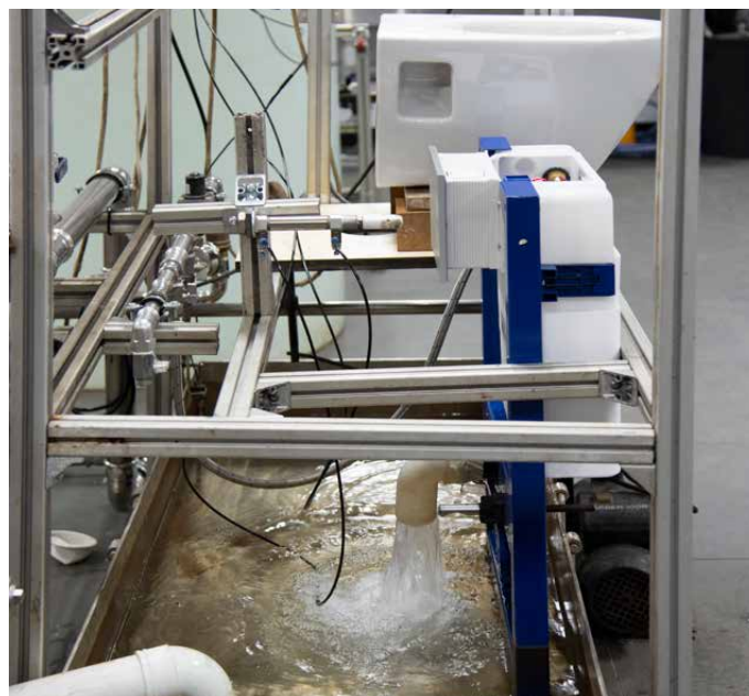
Recycling of water for sanitary ware testing under Water Efficiency Labelling Scheme (WELS).
